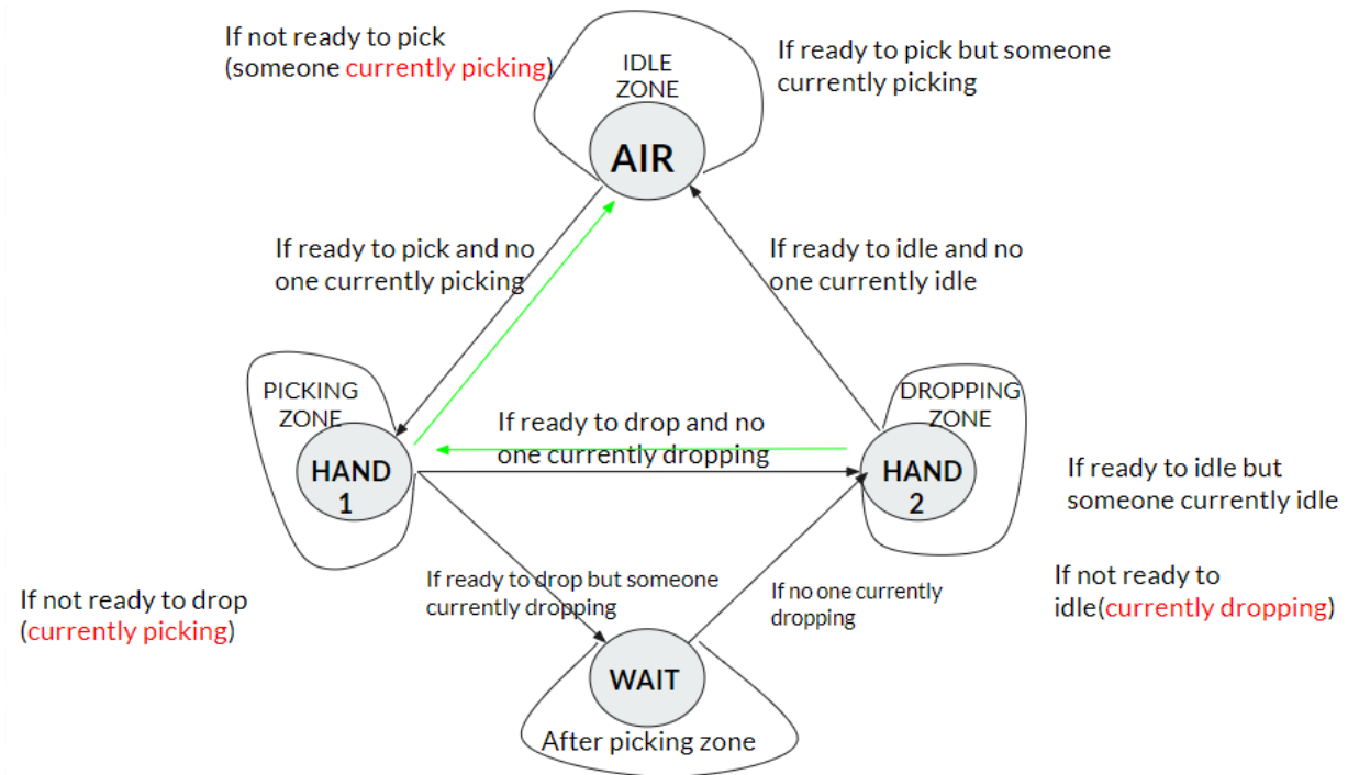
Figure 4.10 Modified scheduling Algorithm for the swarm
