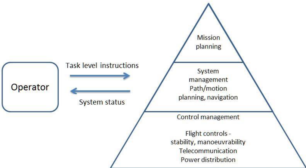
Figure 3.8 Autonomous control basics
