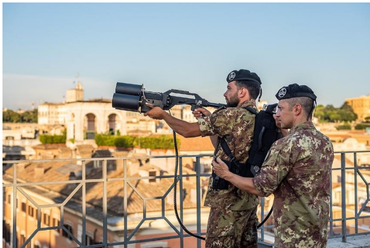
Figure 3.10 Italian Army soldiers of the 17th Anti-aircraft Artillery Regiment "Sforzesca" with a portable CPM-Drone Jammer in Rome
